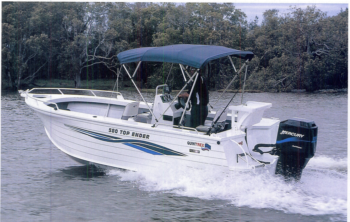
The Quintrex Top Ender's Maxi 2 transom provides a lot of lift and combined with flotation makes it suitable for four and two-stroke outboards.
